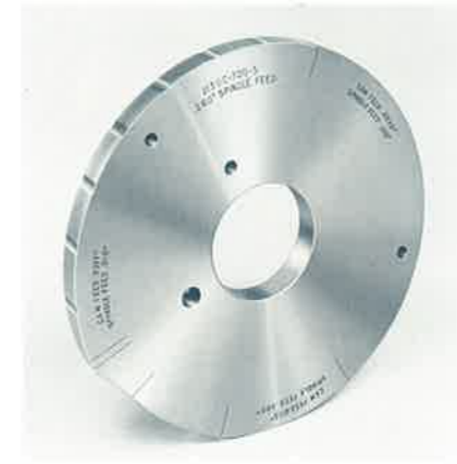
Roughing cam, showing relief portions to permit coolant to enter grinding areas as roughing progresses.
