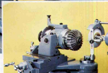
Corner radius grinding of milling cutter
